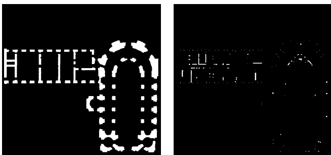
Fig. 3. Walls detected in the floor plan: (left) main walls; (right) dividing walls.
