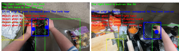
Figure 4. Using the masks provided by VISOR Kitchens, we define the intersection between the object and the hand bounding boxes as the center of the interaction. We show in yellow the bounding box of the non-interacting objects, in green the bounding box of the hands and in blue the bounding box of the interacting object.
