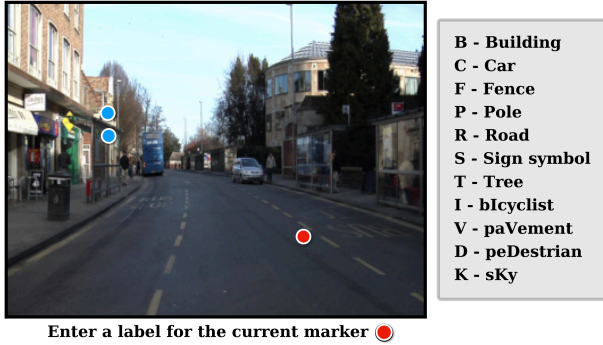
Figure 3: PIXELPICK mouse-free annotation tool. The annotator classifies the highlighted point (in red) by pressing the keyboard character of the corresponding class for the dataset. The tool then highlights the next pixel proposal and the process repeats. Note that the task involves classification, but not localisation.
