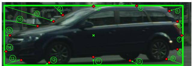
Figure 3: The vertex selection strategy: we trace lines at regular intervals in the bounding box, starting at the top left corner and going clockwise. The selected vertex is the first point on the line within the instance mask when going from the bounding box toward the center. The interval changes depending on the number of vertices used in the method.
