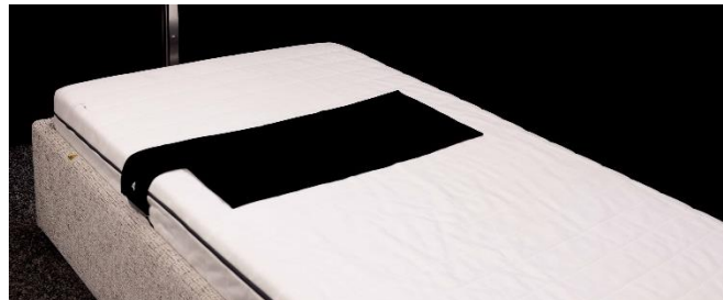
Figure 3. ISABel I, a standard bed with a single eight-channel force sensor.
