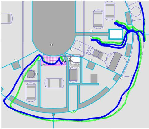
Figure 14. Trajectories estimated by the EKF (dashed green line) and the map-matching trajectory obtained by applying the particle filter on the EKF output (solid blue line).
