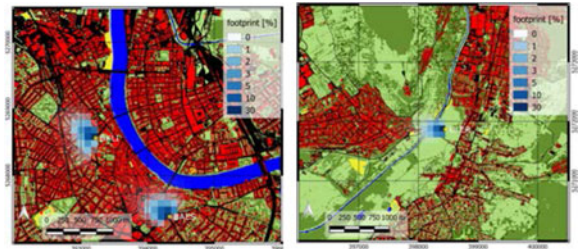
Fig. 6. Weighted footprints for August 30, 2015, satellite overpass (11:00 UTC+1). Left: Urban flux towers BKLI and BAES. Right: Rural/suburban flux tower BLER. Reference system is UTM 32N.
