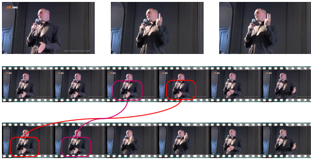
Fig. 7. The Varoufakis video copy-move. Three versions of the same video appeared on the web, with radically different content, as per the sample frames shown on the top row. With reference to the video on the left where the arm is down, a copy-move detector revealed that a sequence from one video (second row) was temporally flipped and copy-moved onto another one (bottom row). For the other two videos the detector was not able to tell apart the pristine from the forged one, since the discriminative region was too small.
