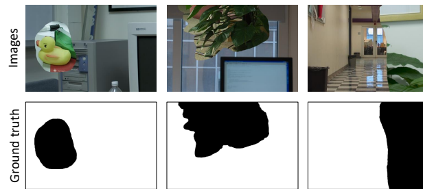
Fig. 13. Examples from the Columbia dataset. Top: images with splicing, bottom: ground truth. In all cases the inserted region is very large and obviously detectable.
