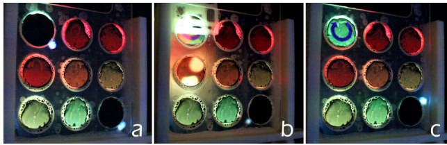
Figure 6. (a) Music is being played for two popped films (b) the user reformes the soap film with a slider on top-left corner. (c) The music mapped on the recreated film has been stopped (spinning circle disappeared).
