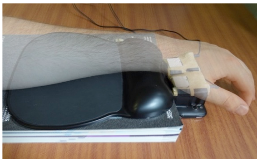
Figure 2: Experimental setup with Peltier elements under the palm and the padded armrest for comfort.
