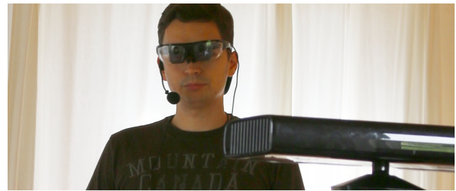
Figure 4. System setup: user wearing the HMD and microphone (far plane), and a Microsoft Kinect oriented towards him (near plane).
