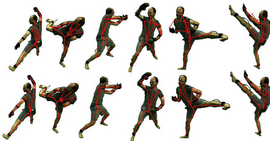
Fig. 6. Freestyle sequence for (ICP) top row and bottom row (proposed). The segmented image is shown with the reconstructed skeleton overlaid.
