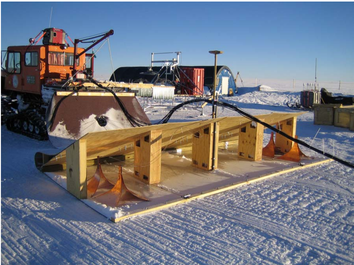
Fig. 3-14. Transmit antenna array with 4 TEM horn antennas. The transmit array really consists of two pairs of antennas which operate in parallel for improved return loss characteristics.
