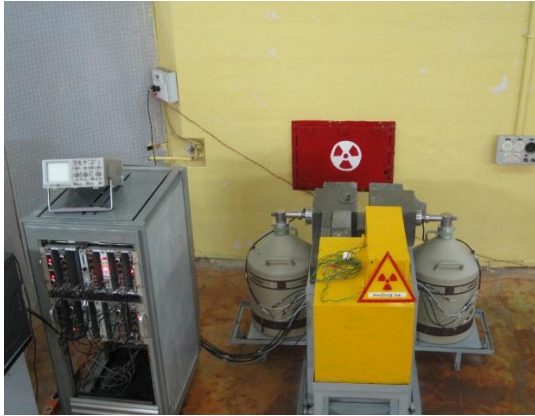
Fig. 8. Event-event coincidence spectroscopy system.
