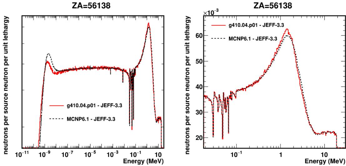
FIG. 2. Energy distributions integrated over all angles of the secondary neutrons obtained with Geant4 and with MCNP6 using JEFF-3.3 for  $^{138}\text{Ba}$  (see the text for more details). The right panel is a zoom of the left panel. In this case  $d_1 = 1.13\%$ ,  $d_2 = 1.64\%$  and  $\chi_v^2 = 2.9$ .
