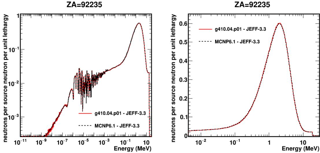
FIG. 4. Energy distributions integrated over all angles of the secondary neutrons obtained with Geant4 and with MCNP6 using JEFF-3.3 for  $^{235}\text{U}$  (see the text for more details). The right panel is a zoom of the left panel. In this case  $d_1 = 1.80\%$ ,  $d_2 = 1.13\%$  and  $\chi^2_\nu = 3.2$ .
