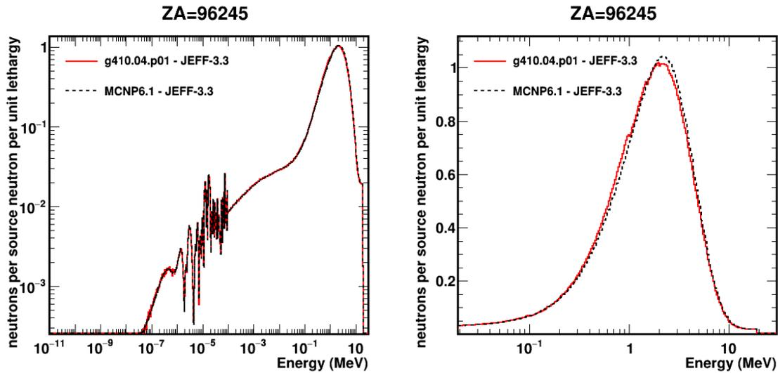
FIG. 3. Energy distributions integrated over all angles of the secondary neutrons obtained with Geant4 and with MCNP6 using JEFF-3.3 for  $^{245}\text{Cm}$  (see the text for more details). The right panel is a zoom of the left panel. In this case  $d_1 = 2.81\%$ ,  $d_2 = 3.74\%$  and  $\chi_v^2 = 72$ .
