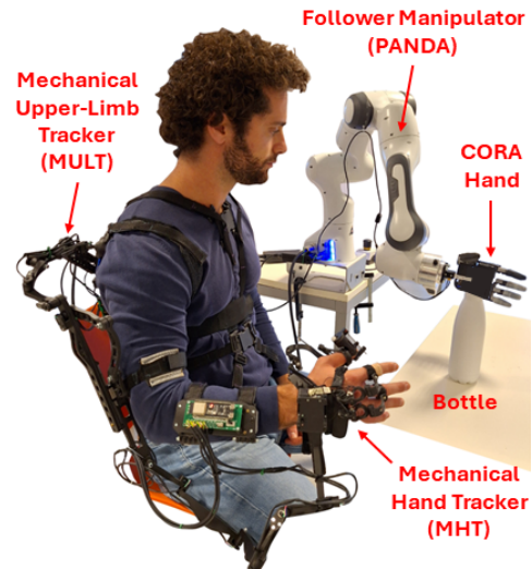
Fig. 2. Experimental setup arranged for a pick-and-place telemanipulation scenario.
