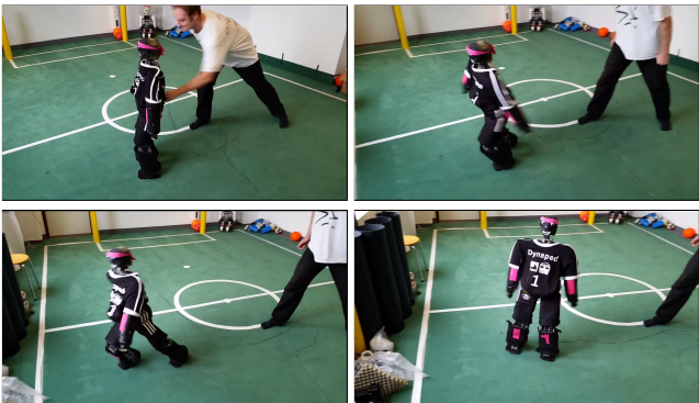
Fig. 1 Push recovery with bipedal robot Dynaped.
