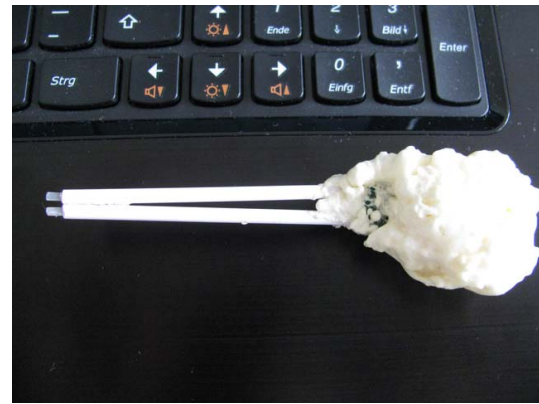
Fig. 2. Thermocouple design with foam coat for thermal insulation of the cold junction.
