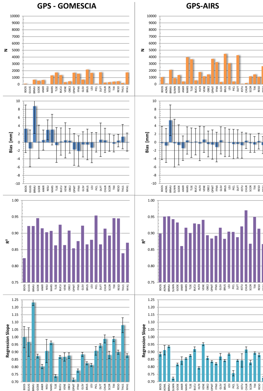
Figure 12. Column bar plots of scatter plot properties (count N , bias, R^2 and regression slope) of the different satellite instruments versus GPS for the selected sites. Sites are ordered with increasing latitude. The error bars represent the SD of the differences (bias panels) and the one-sigma uncertainty estimate of the regression slopes.
