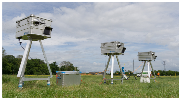
Figure 1. Swiss miniDOAS scheme and field set-up of three instruments (retro-reflectors and shutter not shown).
