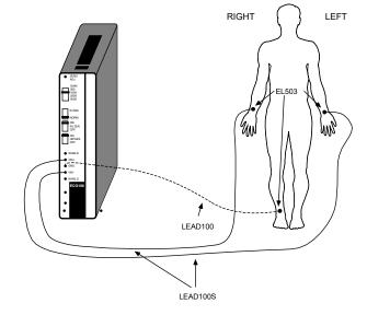
This figure shows the electrode connections to two ECG100C modules for recording a standard **two lead ECG** (Lead I and Lead III). Although only two channels are directly acquired, Lead II can be computed (either on-line or after the fact) by summing Lead I and Lead III. For this setup, the GND input on Lead I is internally connected to the GND input on Lead III, and the VIN+ on Lead I is connected to the VIN- on Lead III via a JUMP100C jumper lead.
