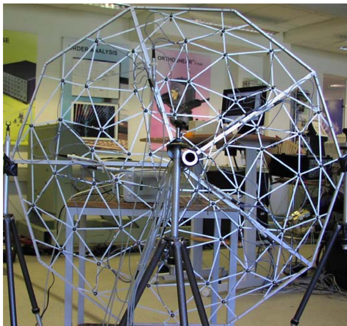
Figure 8: Picture of the measurement set-up. The small loudspeaker can be seen behind the 60-element Pizza Array, just below and to the left of the center.
