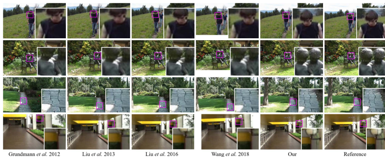
Figure 7: Visual comparison with offline approaches [9, 17, 19, 29] in terms of zoom-in effect. Pink bounding boxes of the same size are magnified to show image regions at the same respective locations. Our approach shows the least amount of distortion and zoom-in effect. Please see our supplementary video for visual results.
