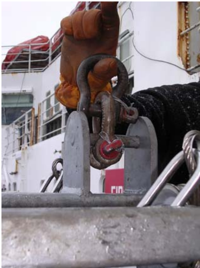
Figure 13: Photo showing correct configuration of shackles for attaching the box core yoke hook to the axle.
