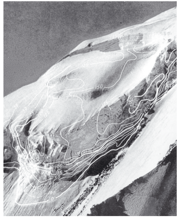
Fig. 21. Motion of the serac of Weisshorn glacier, obtained from a photogrammetric analysis of terrestrial pictures taken prior to the 1973 rupture (see also Fig. 6). The deformations are concentrated in the vicinity of the glacier bed, where the formation of the cracks is concentrated (VAW, unpublished).
