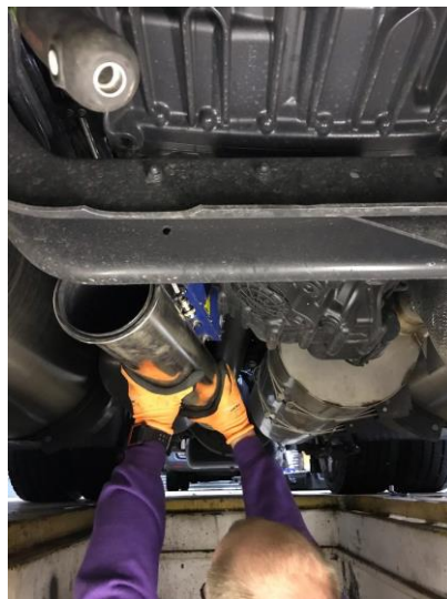
Figure 16: Fitting of PEMS equipment
