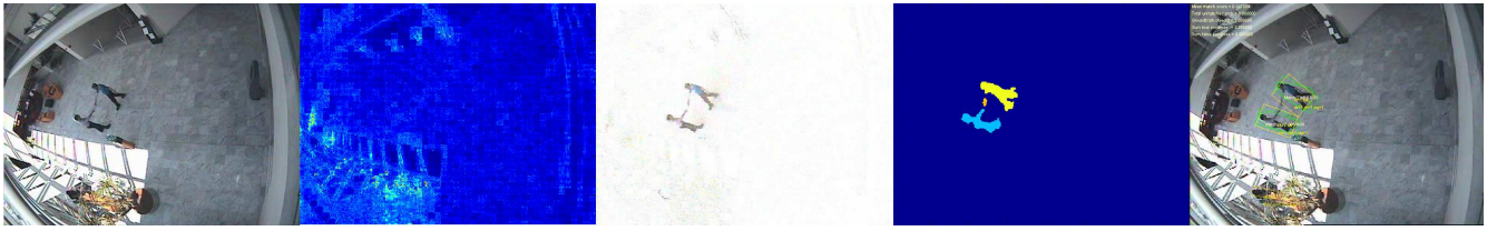
Fig. 13 Tracking results (from left to right): Original frame; Model of the background variances; Results of background subtraction; Detected blobs after morphological operations; Resulting tracked objects (outlined in green) with ground truth data and results shown in yellow.
