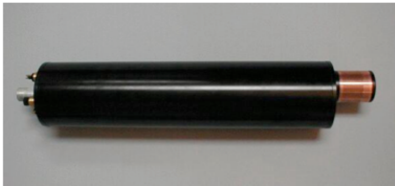
Figure B5. The ISUS Satlantic NO 3 sensor
