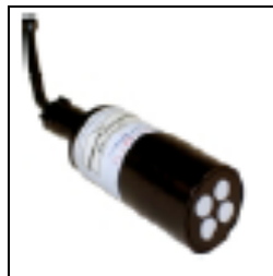
Figure A4: Satlantic OCR-500 Irradiance sensor.
