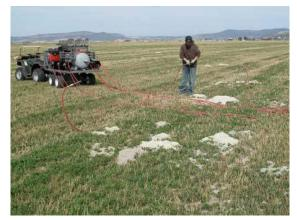
monoxide (CO) gas with the rodents reportedly killed before they escape the burrow. Kohler Co. engines are exclusively used to power the H&M Gopher Control equipment.
