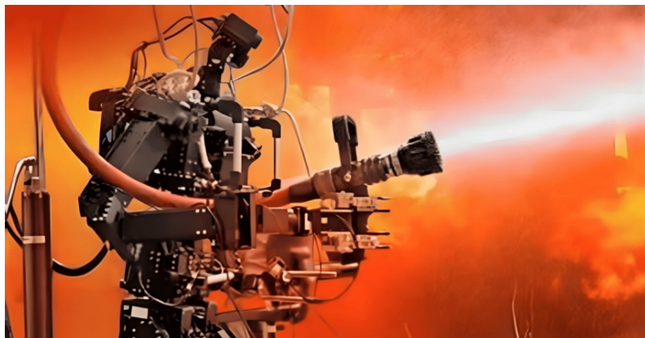
FIGURE 4: Autonomous firefighting robot
