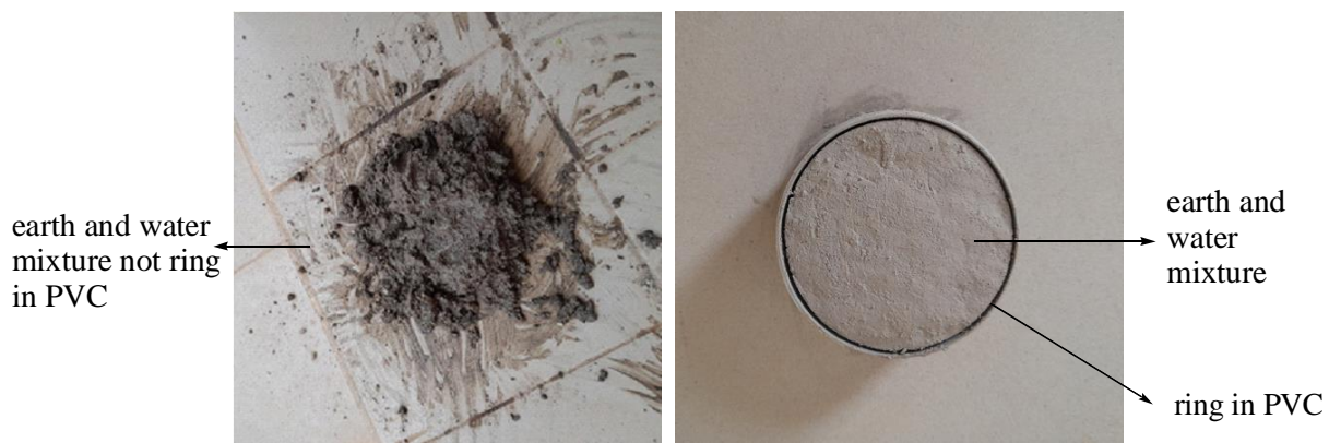
Fig. 5 Sample of raw earth brick crushed and kneaded with water and easy withdrawal from the ring after six (6) days of filling.
