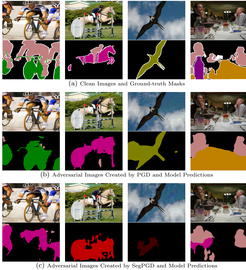
Fig. 3: Visualizing of Adversarial Examples and Predictions on them. SegPGD create more effective adversarial examples than PGD.
