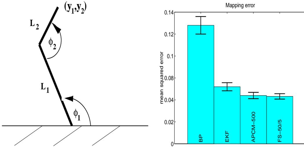
**Figure 4.** **Left:** Schematic illustration of the two link robot arm. **Right:** Mean squared errors on the underlying (unnoisy) transformations (96) and (97). The heights of the bars show average mean squared errors on a regular grid of the input space  $[0.3, 1.2] \times [\pi/2, 3\pi/2]$ .
