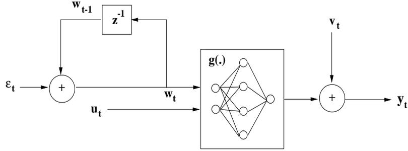
**Figure 2.** Dynamic neural regression model in engineering block form. The  $z^{-1}$  block is a unit time delay. The non-linearity  $g(\cdot)$  is represented by a multi-layer perceptron neural network model. The covariance matrix of the Gaussian disturbance term  $\epsilon_t$  is  $\mathbf{Q}_t$  and the variance of the Gaussian measurement noise  $v_t$  is  $\sigma_{v_t}^2$ .
