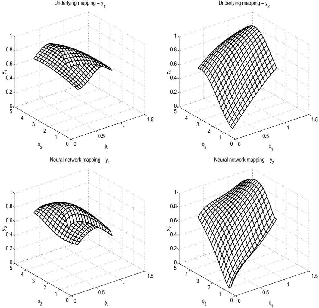
**Figure 5.** Original and neural network mappings after online adaptation with the Fisher scoring algorithm. The top plots show the original mappings (96) and (97) for the input space  $[0.3, 1.2] \times [\pi/2, 3\pi/2]$ . The bottom plots display the neural network mappings evaluated at weight vector  $\mathbf{w}_{1000|1000}^{\text{FS}}$  for the Fisher scoring online learning approach.
