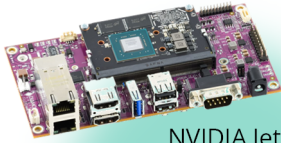
NVIDIA Jetson carriers used in intelligent signage and EV charging stations
