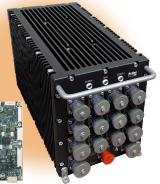
Rugged SBC used in ATR system
