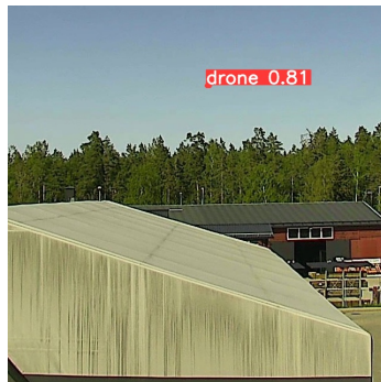
(c) Tiled image from the original image. The model trained with original-size images succeeded in detecting the drone.
