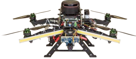
Figure 2.8: UAV used in the following hardware experiments. Notably, the UAV is equipped with a rotating 2D LiDAR (for obstacle perception), an Intel UpBoard for onboard computation, and the ROSflight FCU.
