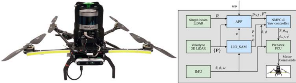
Figure 3.1: 3D-LiDAR equipped UAV, and the complete LiDAR SLAM and local navigation architecture used during experiments.
