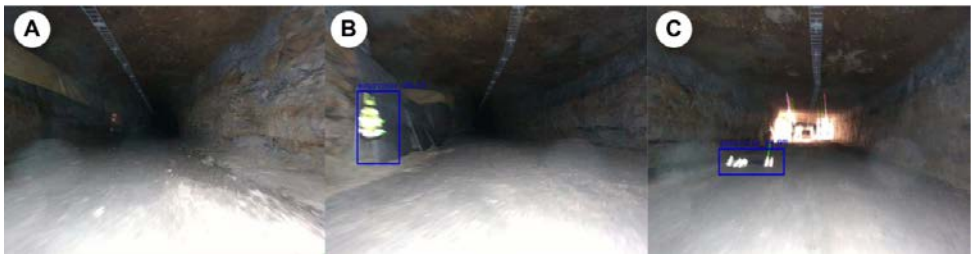
Figure 5.13: COMPRA mission in a wider tunnel at the Epiroc test site. Total mission length of around 200 meters. Detected reflective jackets were placed to mimic "survivor" artefacts.
