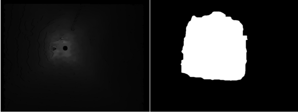
Figure 5.6: snapshots of the DPHR methodology depicting: on the left the extracted centroid (marked black circle) of the open tunnel area and on the right the binarized image of the segmented area with the higher depth values.
