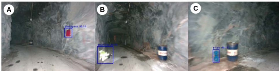
Figure 5.10: COMBRA mission in a curving tunnel environment approximately 3 meters wide. The figure shows the generated map with detected artefacts (top) and snapshots from the onboard camera during the mission (bottom).
