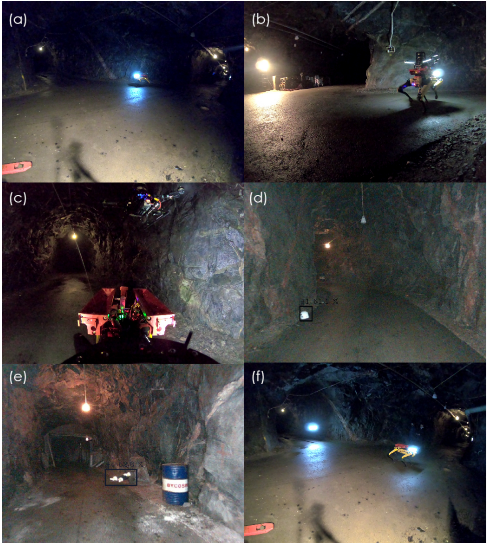
Figure 5.17: Snap shots from the full mission. Spot-UAV system approaching deployment point (top left), deployment point reached (top right), aerial agent take-off (middle left), hard hat detection from onboard camera during COMPRA mission (middle right), survivor detection (bottom left), and aerial agent return to deployment point (bottom right).
