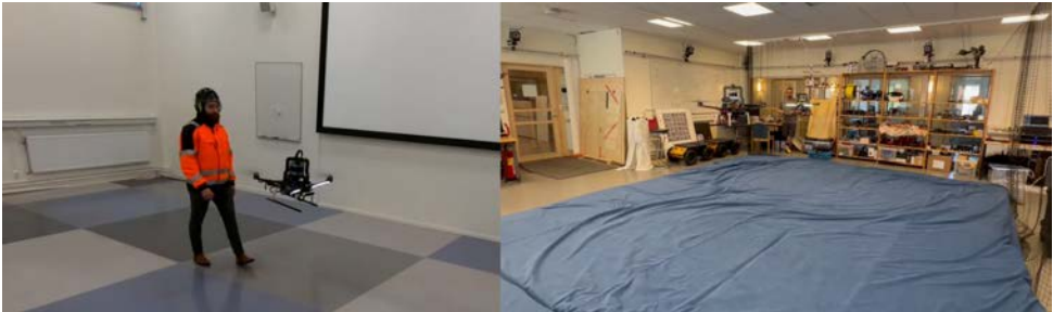
Figure 3.5: Mixed-traffic scenario evaluations. A human worker walks into the operating space of the UAV and avoidance maneuvers are executed (left). Set-up for multi-agent experiment: two large-scale 3D LiDAR equipped UAVs are flying in close proximity and are tasked to swap positions in a confined space (right).
