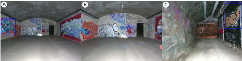
Figure 5.9: Examples of false positive detections during COMPRA missions, which are the reasons for the object validator. The validator rejects these detection hits on the basis of size of the object and the detection confidence.
