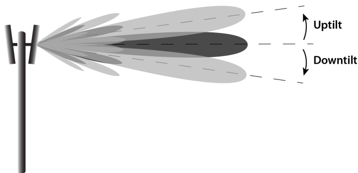
Figure 3.1: Illustration of uptilting and downtilting
