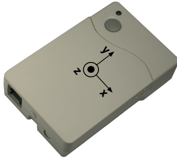
Figure 5: The prototype device with axis orientation notations of the internal acceleration sensor.
