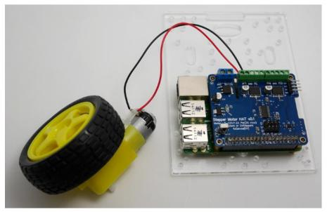
Note: need to external power supply to the motor power supply
