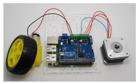
Note: need to external power supply to the motor power supply
