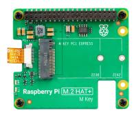
The Raspberry Pi M.2 HAT+ enables you to connect M.2 peripherals such as NVMe drives and AI accelerators to Raspberry Pi 5's PCIe 2.0 interface, supporting fast (up to 500 MB/s) data transfer to and from NVMe drives and other PCIe accessories.
