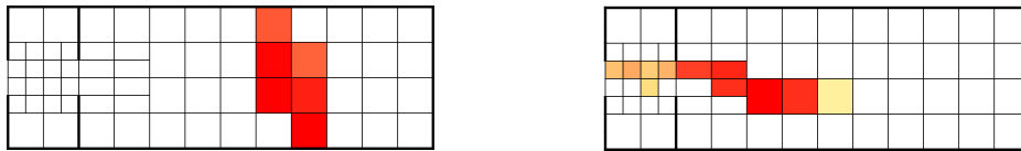
Figure 3. Trajectory reconstruction of a cosmic ray event (left) and of a proton scattered by a 300 keV neutron.
