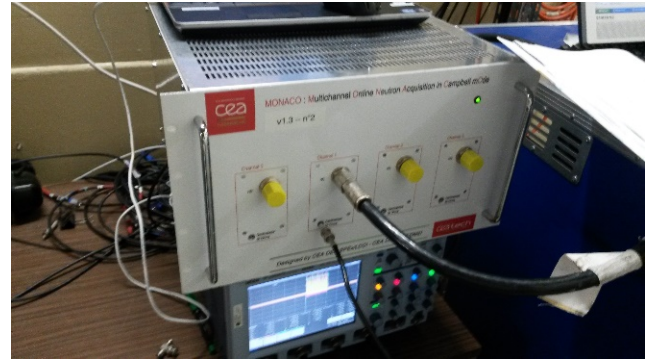
Figure 5 : MONACO prototype electronics.
