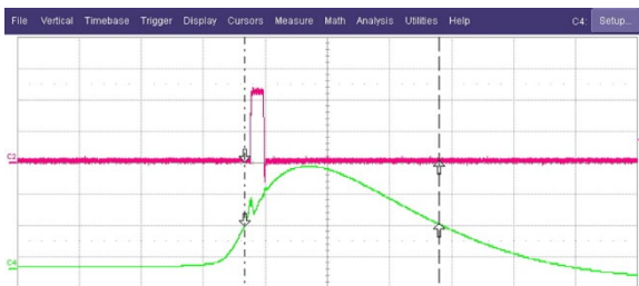
Figure 6 : Average analog signal (green; 50 mV/div) and logical TTL signal (pink; 2 V/div) for the PDT10A module (time base 500 ns/div).
