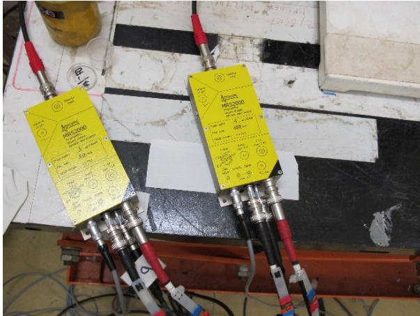
Figure 4 : Mesytec modules (MRS2000-1 on the left and MRS2000-2 on the right).
