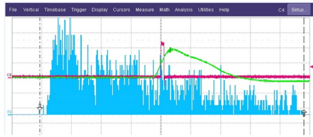
Figure 8 : Pulse height distribution of the analog signal for the PDT10A module starting at 65 mV (3 events/div; 35 mV/div for the horizontal scale).
