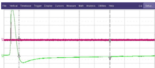
Figure 7 : Zoom on the overshoot observed for the average analog pulse (green; 20 mV/div) of the PDT10A module (time base 5 \mu s/div).
