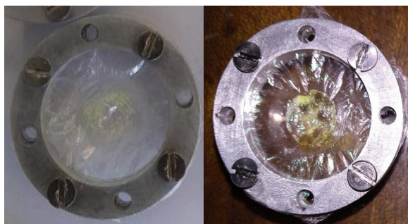
Fig. 1. 1 mg of Natural Sulfur deposited over a disk of 1 cm diameter. Left: target before irradiation, Right: target after 2 continuous days of irradiation with E_{lab} = 3 MeV, I_b = 6 nA proton beam.
