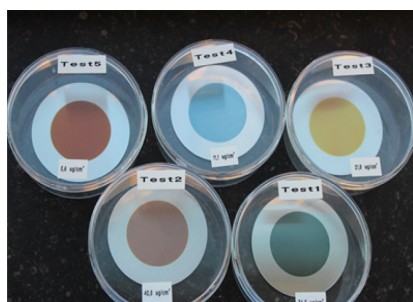
Fig. 2. Pictures five boron test targets prepared at JRC-Geel
