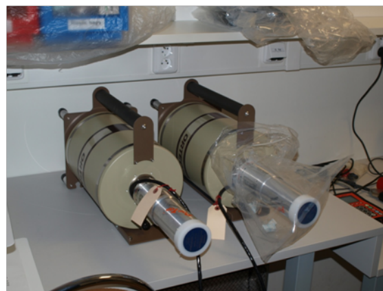
Figure 10. Positionable HPGe detectors
