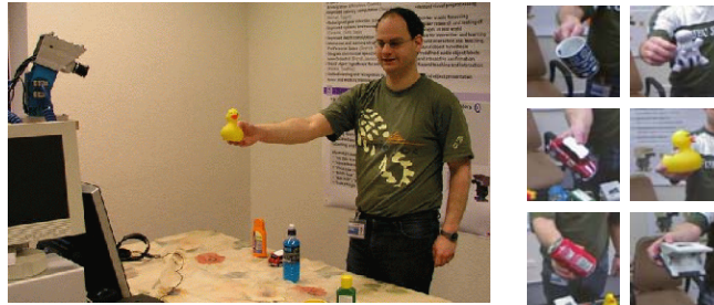
Fig. 1: Presentation scenario for the online learning model of Kirstein et al. The right side shows candidate regions that are passed to the ASDF segmentation stage of Götting et al. and then used to build up an incremental object representation. The system can discriminate freely rotated complex shapes, even if they have similar color structure.
