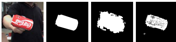
Figure 2: Example for artificial distortion of the ground truth data. From left to right the original image, ground truth \mathcal{G} , distorted hypothesis \mathcal{H} (patchsize s_1 = 12 , shift s_2 = 22 ) and resulting segmentation \mathcal{A} .
