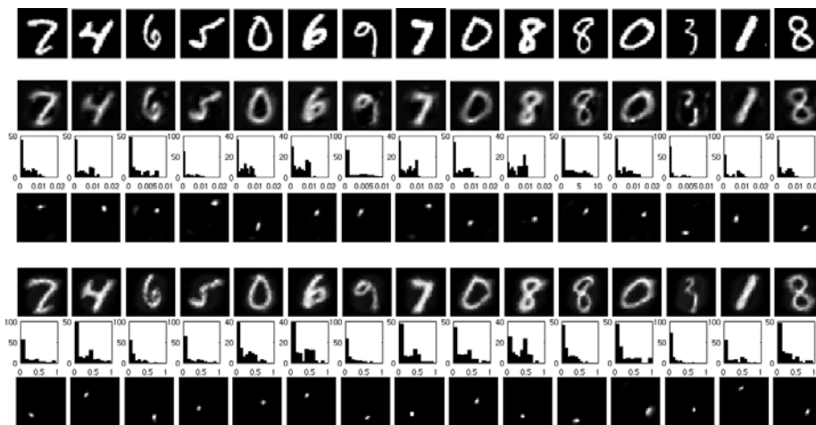
Fig. 2: 15 images from the test set (top row) with reconstructions (2nd row), code histogram (3rd row) and some filters (4th row) performed by the NMFSC. Reconstruction (5th row), code histogram (6th row) and some filters (7th row) performed by the NNSAE.
