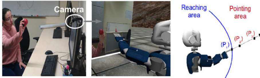
Fig. 1: On the two firsts images, the iCub's simulator tracks and points to a moving ball. On the third image is shown the injectivity characteristic of the mapping from pixel coordinates of both cameras ( \mathbf{u} = (i_L, j_L, i_R, j_R)^T ) to the joint angles ( \mathbf{q} = (\theta_1, \dots, \theta_7) ) of the robot's left arm.
