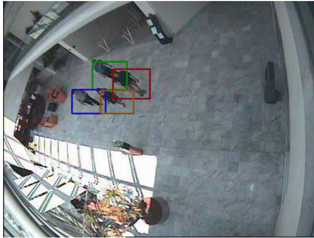
Fig. 2: An image from CAVIAR dataset and the bounding boxes drawn by the tracker.
